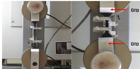
Fig. 3 Uni-axial tension test
