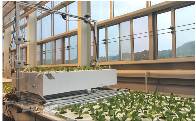
Fig. 2. Sensor location and field view for environmental monitoring in the deep flow technique DFT bed cultivation method.
