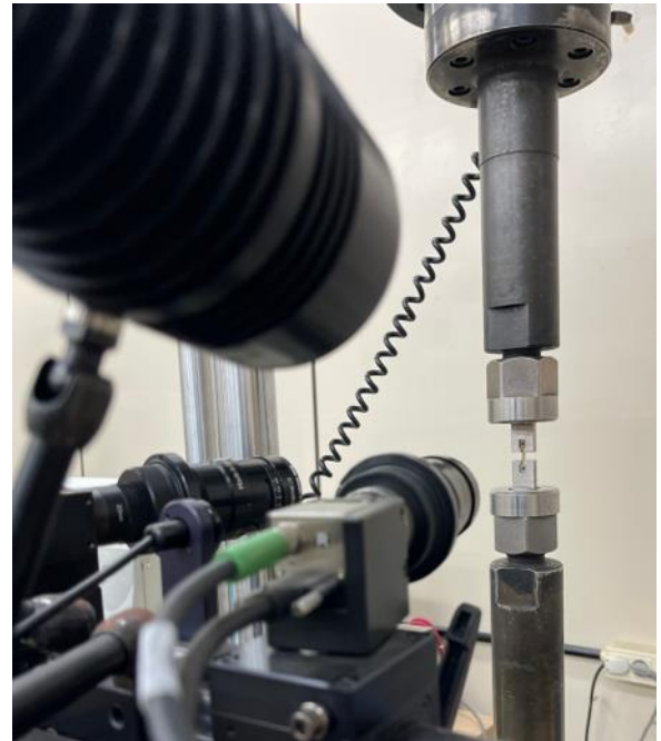
Fig. 2 Uniaxial tensile tests with the DIC technique at room temperature.
