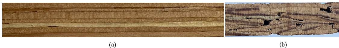
Fig. 2. Illustration view of the planes in PSL. (a) Edge section (7-layer), (b) end section. PSL: parallel strand lumber.
