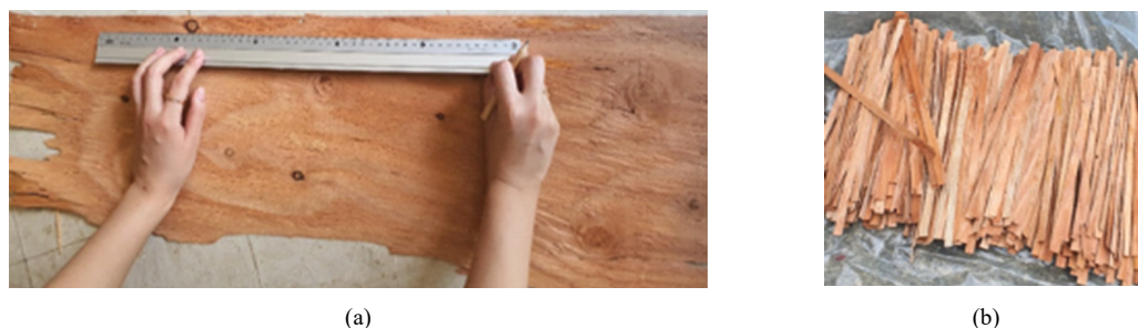
Fig. 1. Illustration of the veneer and strand. (a) Japanese larch veneer sheet, (b) strand from veneer.
