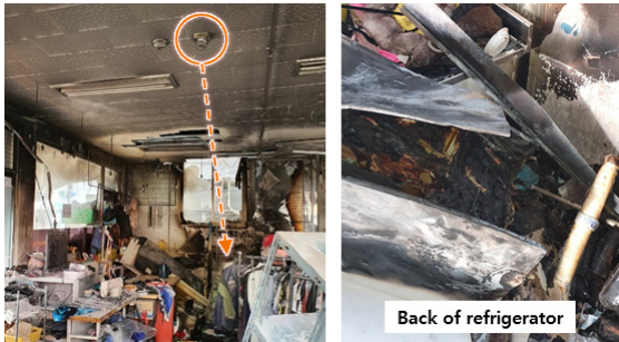
(a) Fire point & detector position
