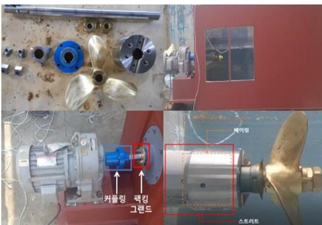
Fig. 6. Rope cutter equipment parts and test water tanks.
