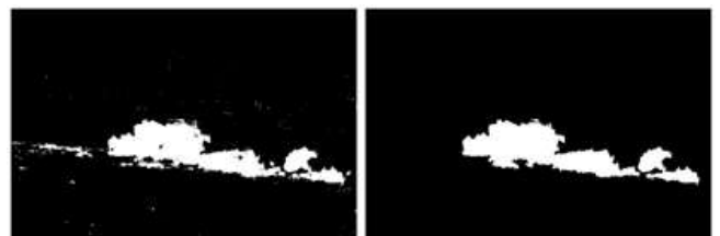
Fig. 9 Binary image obtained from difference image(Left) and binary image with noise removed(Right)
