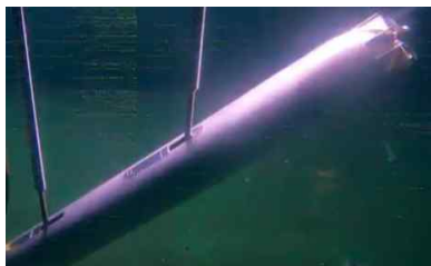
Fig. 6 Underwater snapshot of vertical static test ( \alpha = 35\text{deg} )
