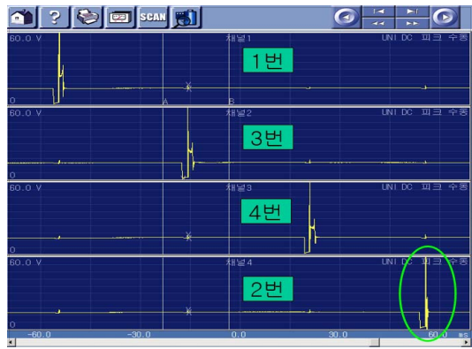
Fig. 8. Ignition pulse example measuring with diagnosis tester
