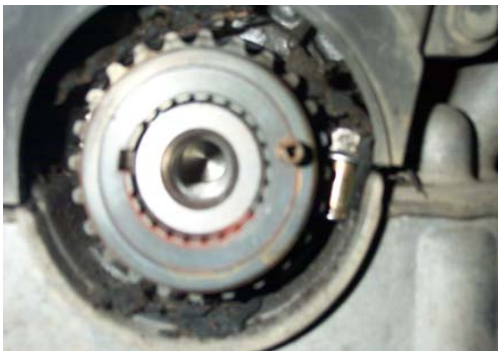
Fig. 4. Front bracket bolt example moving into crank shaft sprocket
