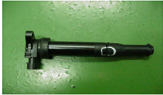
Fig. 7. Leaking example of spark fire in ignition coil
