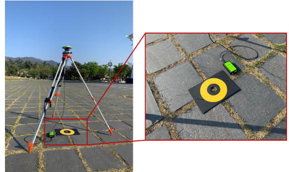
Fig. 3. Example of GNSS surveying with the Alpha receiver
