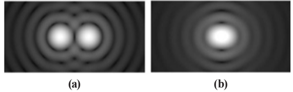
Fig. 6. Airy disk spacing near Rayleigh's criterion
