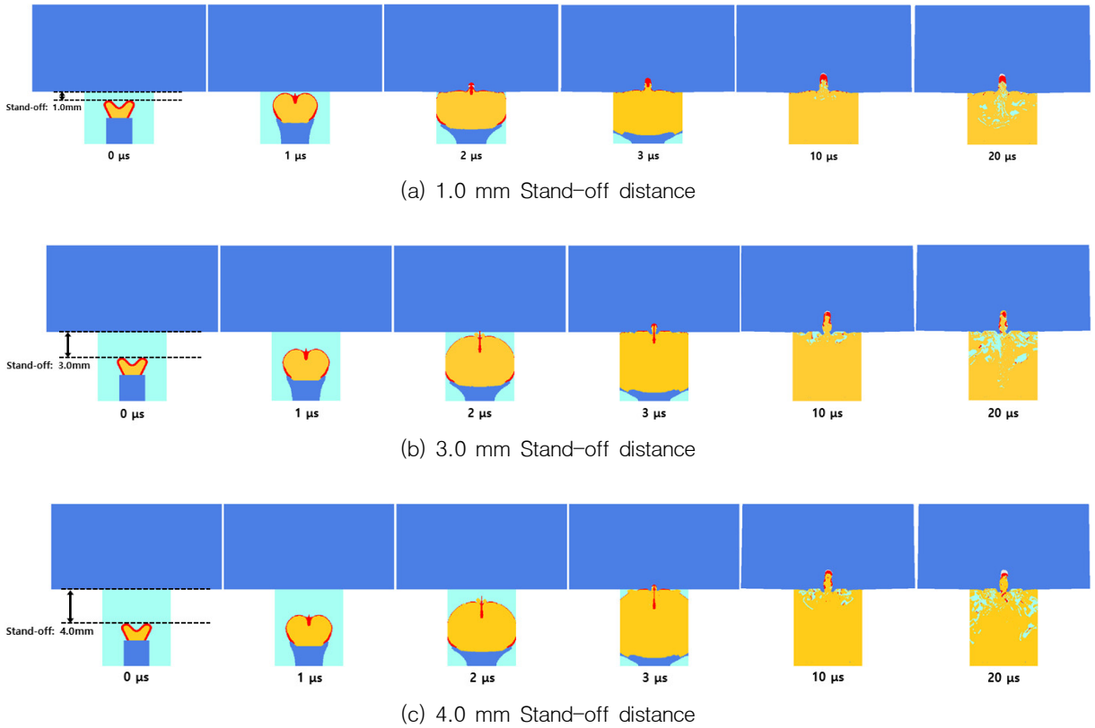
Fig. 9. Numerical results of PLSC specimens with target of Al7075-T6
