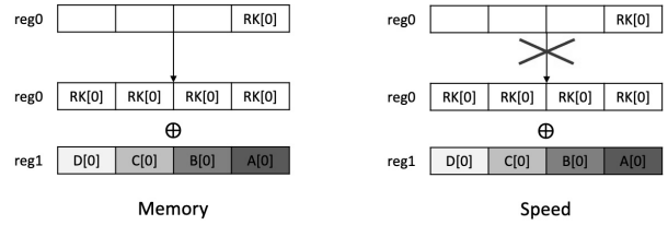
Fig. 9. Memory Optimization AddroundKey(Left) and Speed Optimization AddroundKey(Right)
