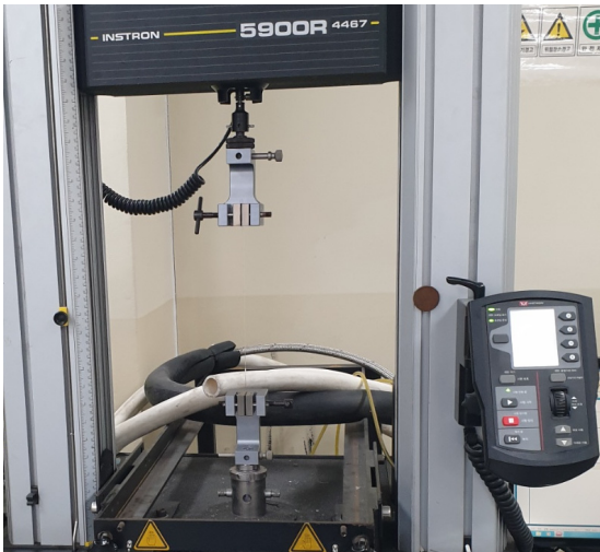
Fig. 3. Tensile testing apparatus for the Nafion 117
