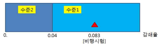
Fig. 4 Evaluation of Flight Test for Phugoid Stability
