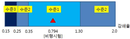
Fig. 5 Evaluation of Flight Test for Short Period Damping Ratio
