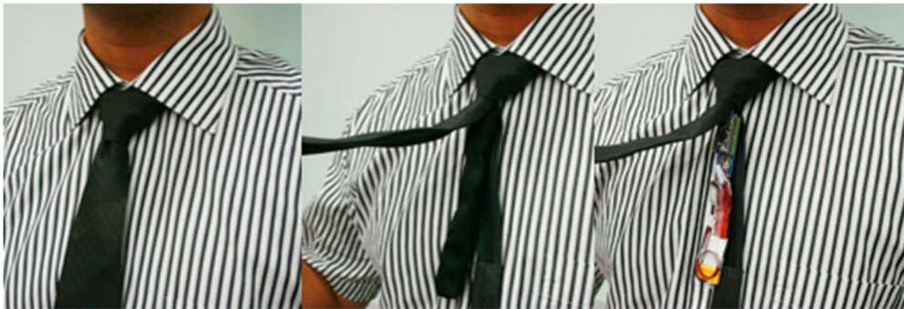
Figure 6. NeckTie prototype with auditory and fragrance actuators and electronic components in a sleeve
