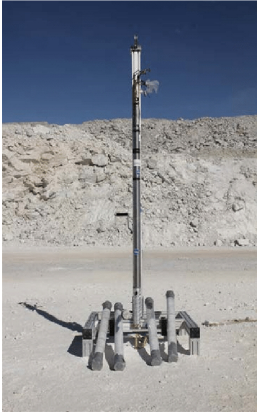
Fig. 5. Auto-Gopher Drill to reach a great drilling depth (Cohen et al., 2016)
