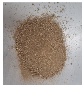
(a) Weathered granite soil
