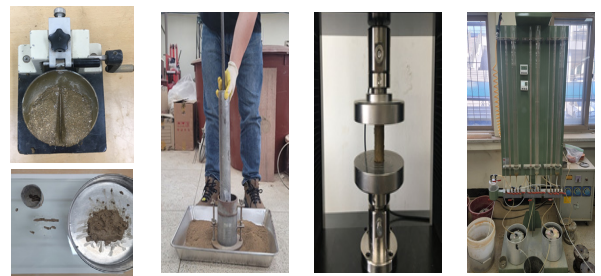
(a) Liquid and Plastic limit test (b) Compaction test (c) Unconfined compression test (d) Permeability test
