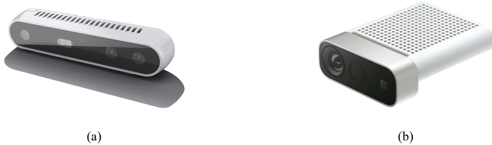
Figure 2. Commonly used Depth Camera (a) Real Sense (D415, Intel, USA); (b) Azure Kinect (Microsoft, USA)
