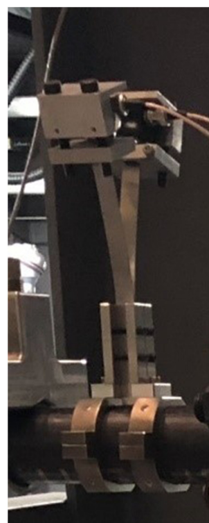
Fig. 5. A waveguide system installed in an area without insulation.
