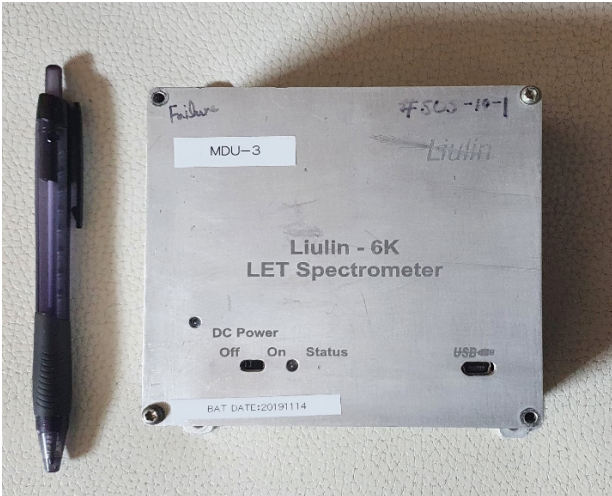
Fig. 2. Liulin-6K LET spectrometer used in the measurements.
