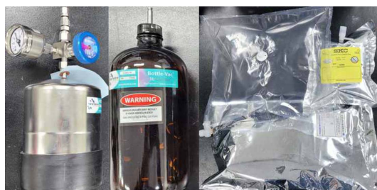
Fig. 1. Gas sample containers used for testing storage stability of the VOCs (from left, Silonite canister, bottle, polymer bags).
