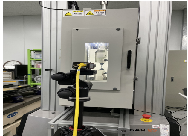
Fig. 2 Experimental set-up for uniaxial tensile testing
