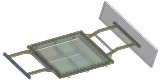
Fig. 3 A head-on impact on the fixed wall(Case 1)
