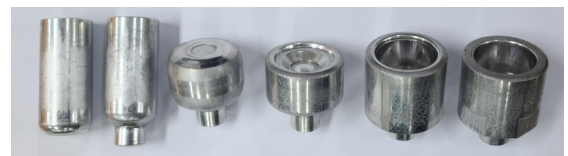
Fig. 8 #10-#60 Cold forming process product
