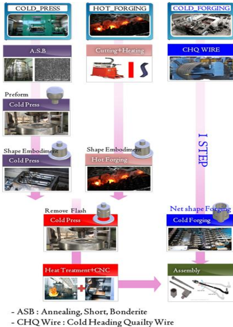
Fig. 1 Inner tie rod socket manufacturing process comparison
