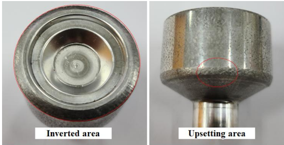
Fig. 10 Check for orange peel and cracks of inverted and upsetting area (#40)
