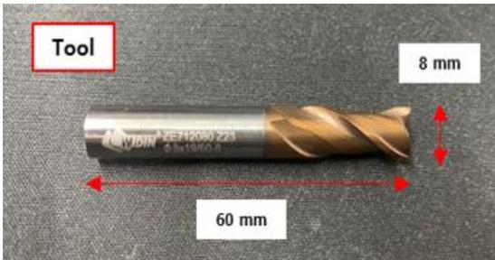
**Fig. 5 Machining Tool**
