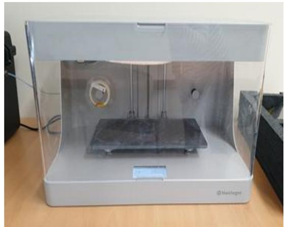
Fig. 1 3D printer for composite materials
