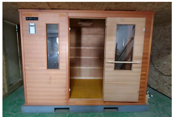
Fig. 1 Heating system experimental device by burying excel pipes on the floor and wall of container house
