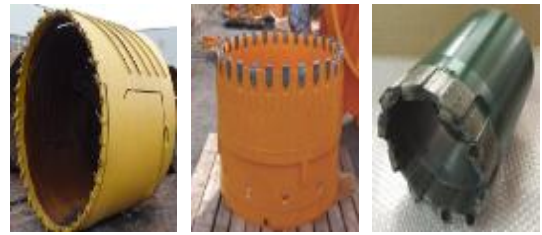
Fig. 3 Example of casing and shoe bit
