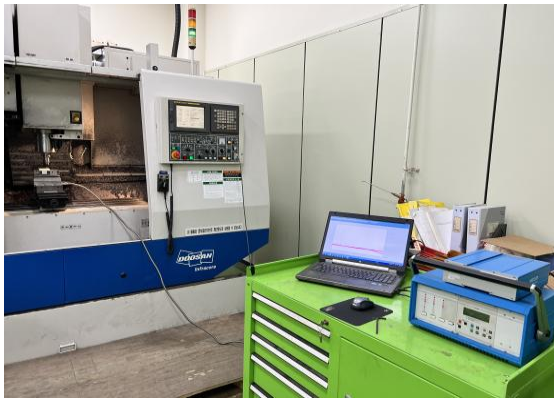
Fig. 3 Experiment setting of grinding force
