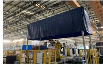
(a) awning shade on the carrier camshaft automation line
