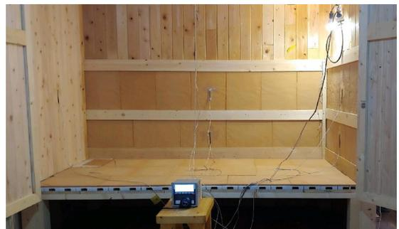
Fig. 1 Heating system experimental device by burying excel pipes on the floor and wall of container house
