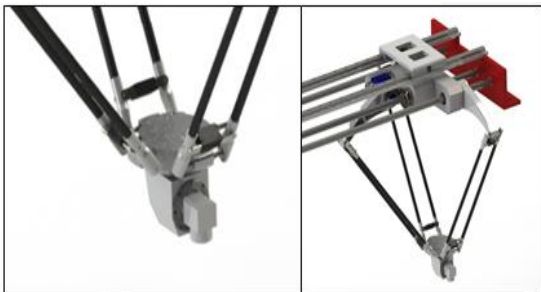
Fig. 3 6-DOF Parallel Robot with a 3-DOF Wrist Mechanism and an Additional Stratght Axis at Its Topodeling
