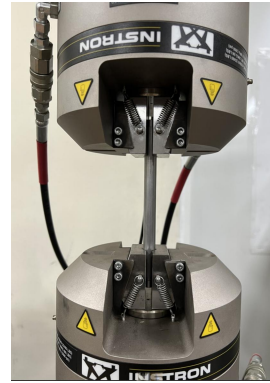
Fig. 4 Photograph of pipe tensile test
