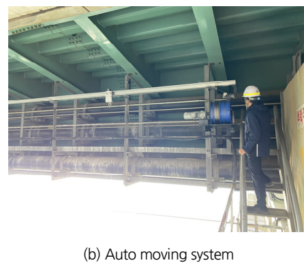
Fig. 5. Current measuring system of NEB control gate (#9)
