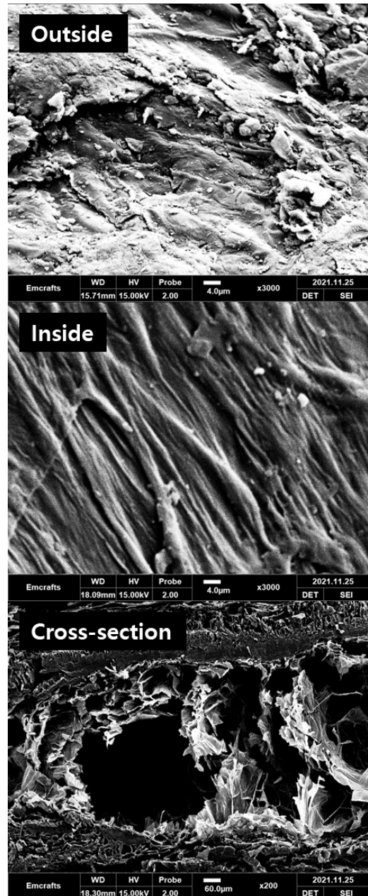
Fig. 3. SEM images of peanut shells. SEM: scanning electron microscopy.
