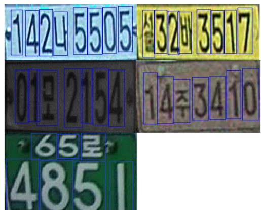
Fig. 7. Examples of character segmentation module.
