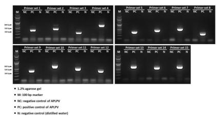
**Supplementary Fig. 2.** Verification of candidate primers designed for *American plum line pattern virus* (APLPV) detection. In total, 15 candidate primer sets were examined by one-step reverse transcription polymerase chain reaction (RT-PCR) assay using APLPV-infected and healthy samples.
