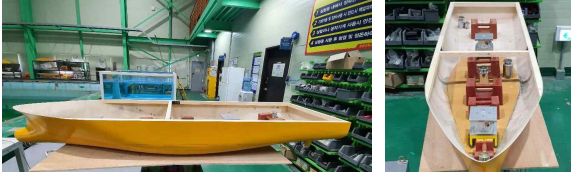
Fig. 6 Inertia test in case 1 (Full loading condition)
