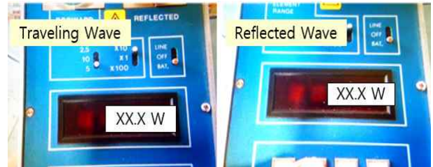
Fig. 12 Traveling and Reflected Waves of RF Cable
