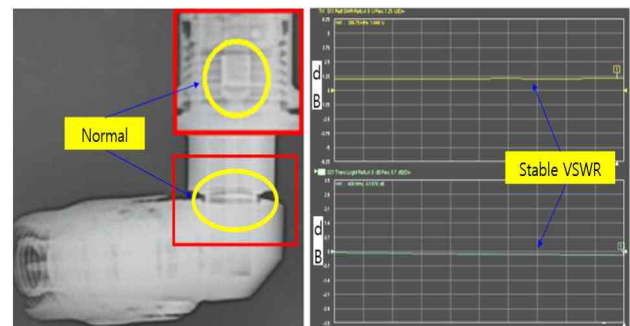
Fig. 9 Results of Disassemble Verification in the RF Cable
