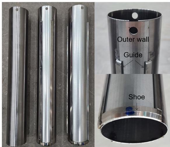
Conventional pile Double wall pile1 Double wall pile2
