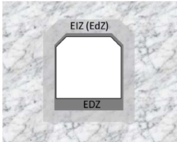
Fig. 3. The concept of excavation-induced damage and influenced (or disturbed) zones (Follin et al., 2021)
