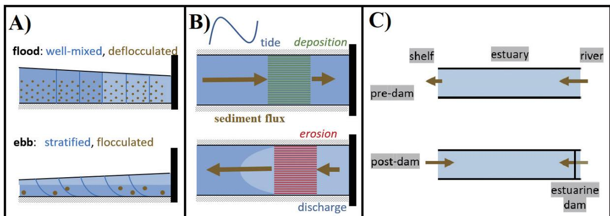
Figure 5. Conceptual diagrams. A) Periodic stratification and flocculation asymmetry after freshwater discharge. B) Competition between landward tidal pumping and seaward river runoff in the inner estuary. In Geum estuary, generally landward tidal pumping is greater. C) Simplified change of sediment flux direction at the mouth from the pre- to post-dam estuary.
