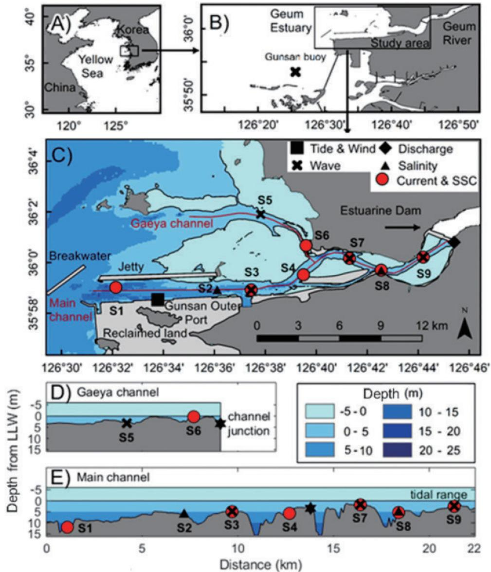
Figure 1. Study area and measurement stations. Depth is relative to a lower low water (LLW) vertical datum. Reprinted from *Marine Geology*, 429, Figueroa, S., Lee, G., Chang, J., Schieder, N., Kim, K., and Kim, S.Y., Evaluation of along-channel sediment flux gradients in an anthropocene estuary with an estuarine dam, 106318, copyright (2020), with permission from Elsevier.
