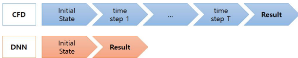
Fig. 1. Difference in the process for estimating resistance performance between CFD and DNN.
