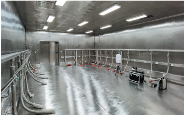
Fig. 6. A laboratory with a background below the natural radioactivity level.
