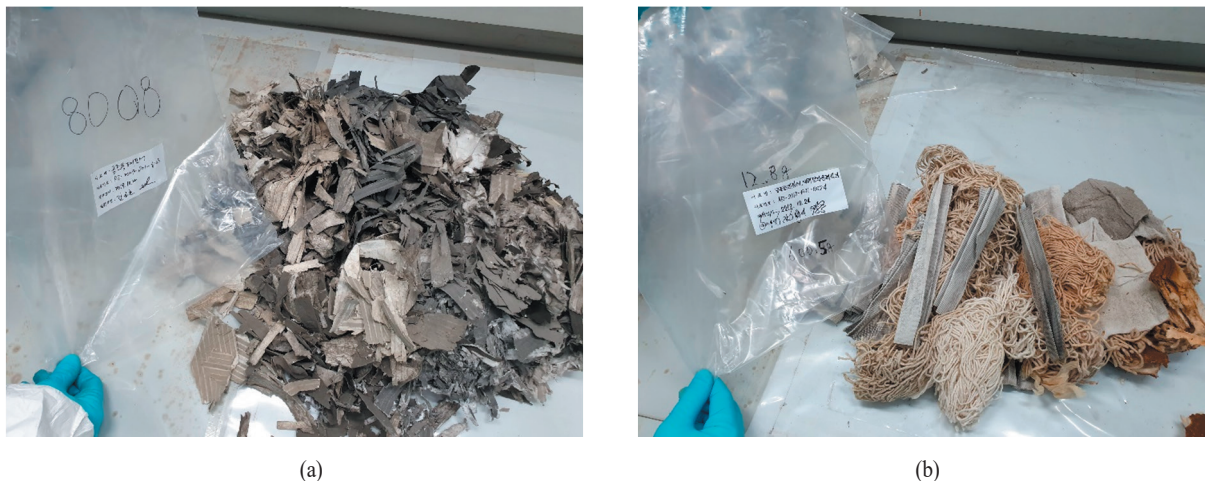
Fig. 1. Photographic images of filter waste samples: (a) air filter, and (b) a mixture of air and water filters.
