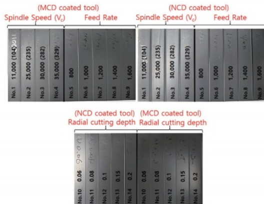
Fig. 3 Machined surfaces according to the cutting
