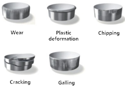
Fig. 3 Most Frequent Failure Mechanisms in Sheet Metal Tooling
