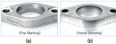
Fig. 2 Product by (a) fineblanking and (b) normal stamping
