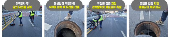
Fig. 7. Calculation and verification method of permittivity constant
