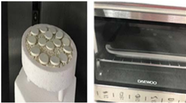
Figure 4. Dried zirconia and dryer (DWO-G13SB; Daewoo, Seoul, Korea).
