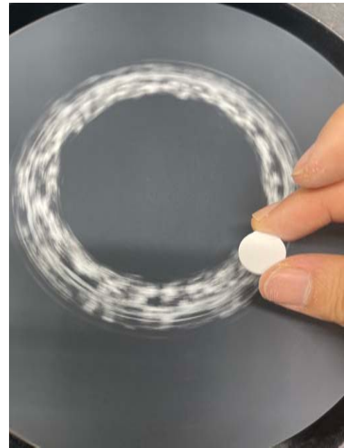
Figure 2. Specimens grinding: 1,500 grit, 2,000 grit.
