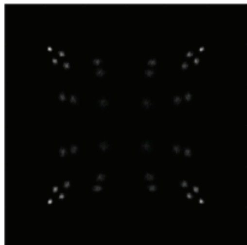
Fig. 3. Flood image acquired through light collected from SiPM generated by each GAGG pixel for look-up table creation.
